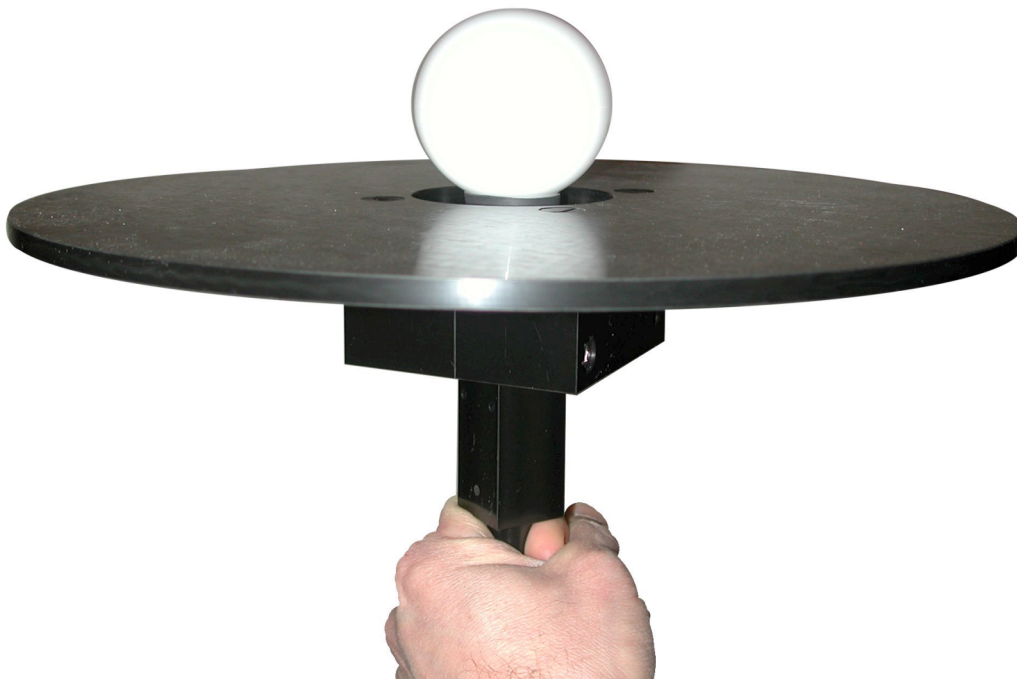
E_0 collector on armored cable
